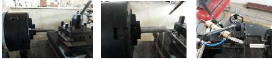
Photo 1,2,3 Dry, wet and VTJA machining
